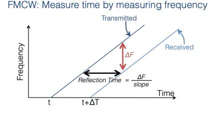
The signal is a **chirp**, where the frequency of the transmitted signal **increases linearly** over time. This means that at any given point in time, the transmitted signal is at a slightly different frequency compared to the reflected signal (because of the delay caused by the round trip)
