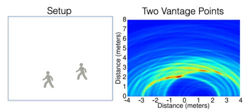
When the system uses **two vantage points**, it can better disambiguate the direct paths of the two walking users by combining the data from both vantage points. This results in a clearer, more accurate representation of each person's movement, as it helps to separate the actual reflections from the **multipath effects**
