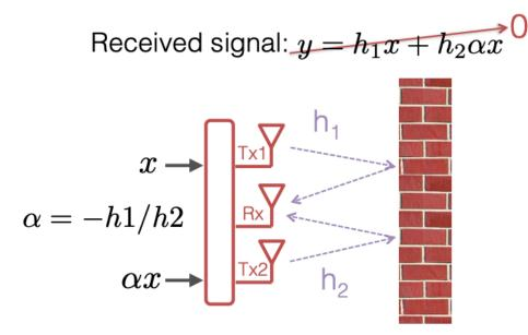
Two transmit antennas and one receive antenna, and set
