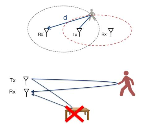
• **Static Multipath**: When tracking a moving person, multipath reflections occur because the transmitted signal reflects off various objects (e.g., furniture) before reaching the receiver
