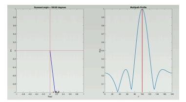
• If the guessed angle is correct, the phase differences are properly corrected, and the signals from the antennas will align, resulting in a large sum
